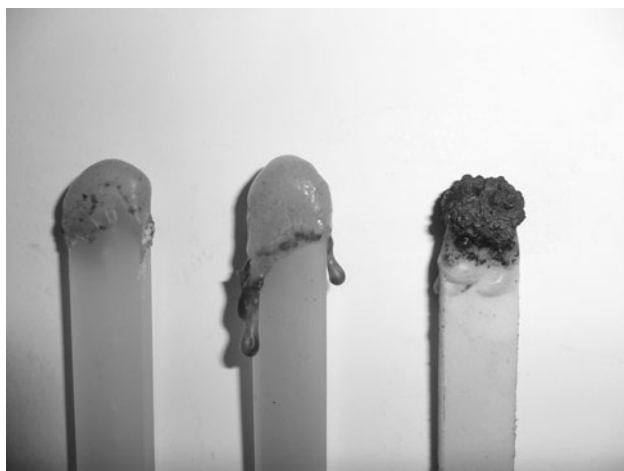
Fig. 2 Digital picture of samples after combustion (left to right PP, APP-PP, IFR-PP)
